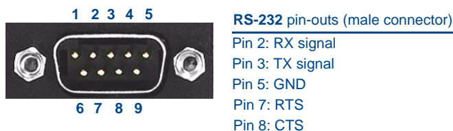
FIG. 6 RS-232 (DB9 - Male) Connector Pin-outs
