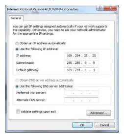
FIG. 2 SETTING A STATIC IP ADDRESS
