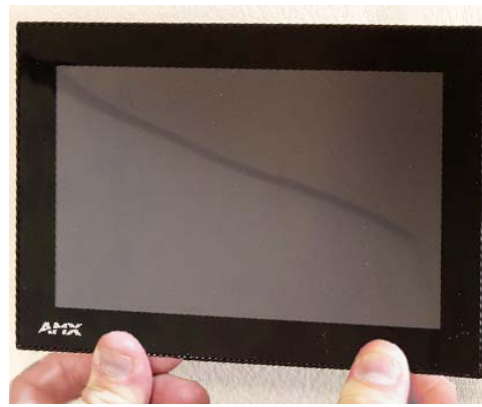
FIG. 8 LOCKING DOWN THE BOTTOM OF THE TOUCH PANEL ONTO THE BACK BOX.
