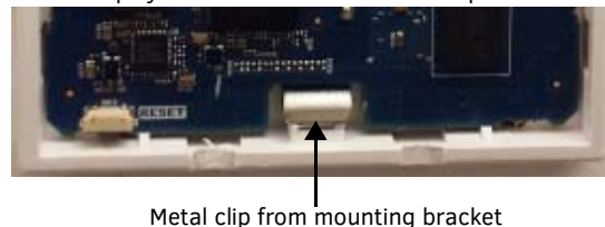
FIG. 27 Metal clip from mounting bracket locking device frame onto bracket
