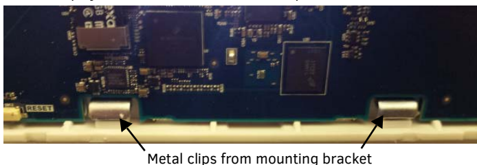
FIG. 26 Metal clips from mounting bracket locking device frame onto bracket
