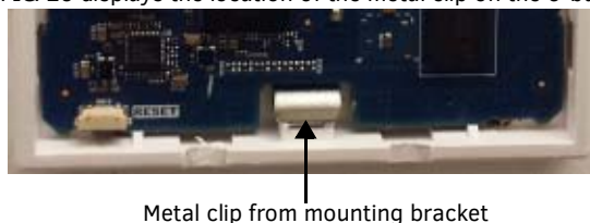
FIG. 20 Metal clip from mounting bracket locking device frame onto bracket
