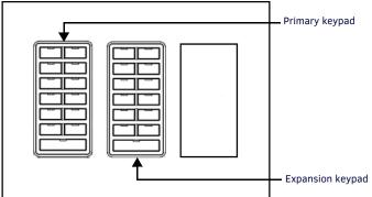
FIG. 3 INSTALL THE KEYPADS IMMEDIATELY ADJACENT TO EACH OTHER IN A 3-GANG BACK BOX NOTE: When the ribbon cable is connected, touching or moving the ribbon cable can cause a temporary disruption in communication causing the keypads to temporarily go offline and return to service within 25-45 seconds of the initial break. Once the keypads are mounted and the ribbon cable is stable, no disruptions should occur.
