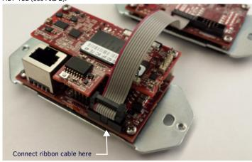
FIG. 2 DAISY-CHAIN CONNECTION BETWEEN THE MET-13E AND AN ETHERNET EXPANSION KEYPAD NOTE: If you are installing a single expansion keypad into a 3-gang back box, install the expansion keypad in the space immediately adjacent to the primary Ethernet keypad (see FIG. 3). Daisy-chaining is supported across a distance of 4" (101.6 mm).
