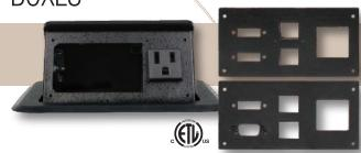
A smaller tilt top style table box for AV/IT Applications. The box has one integrated UL-Rated AC receptacle and ships with two different connector plates (HDMI or DisplayPort connectors, HD-15 connector, and keystone connectors). Our full line of Simple Solutions (SS) keystone snap-in connectors and panel mount HDMI & DisplayPort dongles can easily be used with the TB-AVAC.
