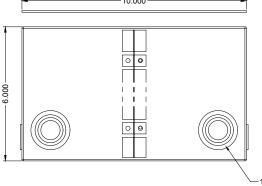
10.000 -1/2" AND 3/4"COMBINATION 1/2". 3/4", 1", AND 1-1/4" COMBINATION KNOCKOUTS (1) PLACE TYPICAL ON OPPOSING SIDES KNOCKOUTS (2) PLACES TYPICAL ON
