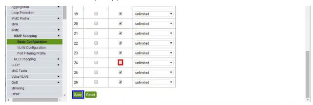
Uncheck the Fast Leave box for ports connected to extended switches.
