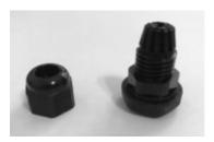
Take plug portion, fit it into mounting hole in enclosure and screw on cap, one rotation, to hold plug in place.
