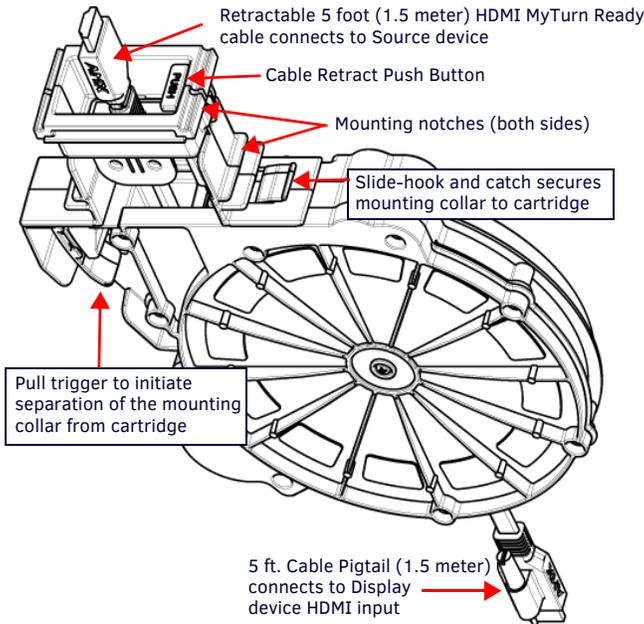
FIG. 1 HPX-AV102-HDMI-R HDMI-R MODULE WITH RETRACTABLE CABLE
