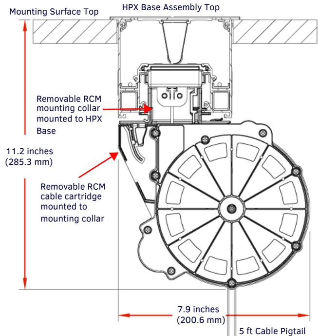
FIG. 8 RCM MODULE (INSTALLED IN AN HPX BASE) - DETAILED DIMENSIONS
