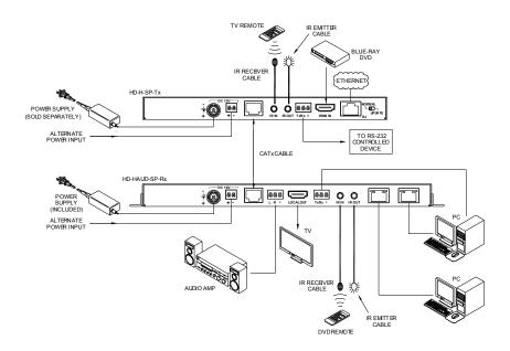
**NOTE:** It is only necessary to power one side (Tx or Rx)
