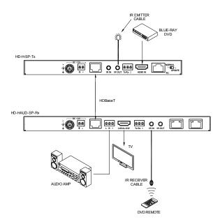
The HD-H-SP-Tx Transmitter is shown in the illustrations throughout this manual. Please note that any of the FSR 100m HD transmitters may be used with the HD-HAUD-SP-Rx Receiver.
