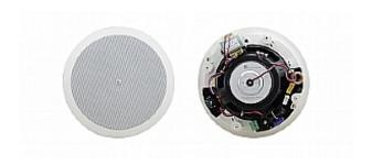
The Galil 8–CO is a pair of two-way, open-back,  $8\Omega$  speakers designed for mounting in the ceiling. The speakers feature a multi-tap power transformer for selecting  $8\Omega$  or 70V/100V power settings suitable for array installation.
