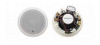
The Galil 6–CO is a pair of two-way open-back  $8\Omega$  speakers designed for mounting in the ceiling. The speakers feature a multi-tap power transformer for selecting direct  $8\Omega$  (bypassing the transformer) or 70V/100V power settings suitable for array installation.
