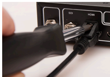
Connecting HDMI Input Cable
