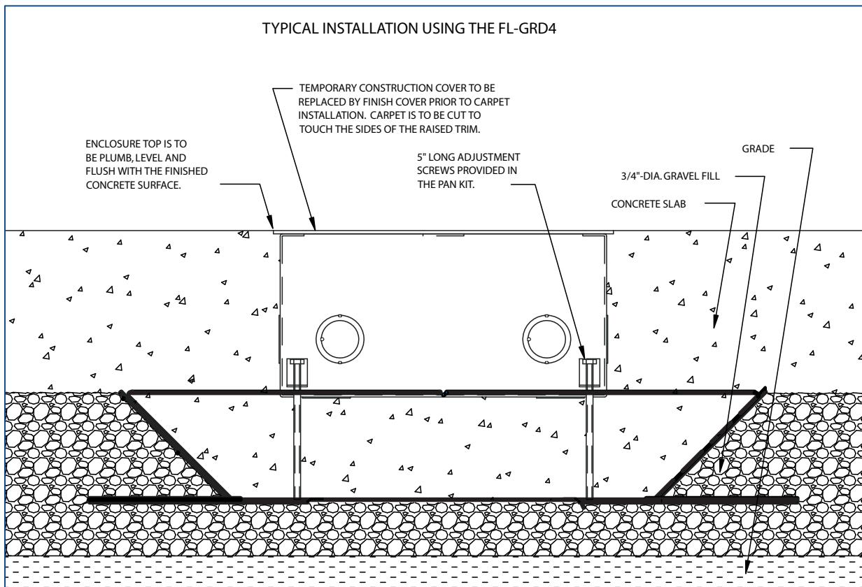
**CONCRETE PAN ASSEMBLY: FL-GRD2 / 4**
