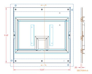
STYLE MODEL NUMBER DESCRIPTION COVER WITH 1/4" BRASS CARPET FLANGE 1 FL-640P-BLP-C (LIFT OFF DOOR) COVER WITH 1/4" SQUARE BRASS CARPET FLANGE (LIFT OFF DOOR) FL-640P-BSQ-C 2 COVER WITH 1/4" ALUMINUM CARPET FL-640P-SLP-C FLANGE (LIFT OFF DOOR) COVER WITH 1/4" SQUARE ALUMINUM CARPET FLANGE (LIFT OFF DOOR) 2 FL-640P-SSQ-C COVER (NO FLANGE) WITH HINGED DOOR 3 FL-640P-BLK-C IN BLACK SANDTEX COVER (NO FLANGE) WITH HINGED DOOR FL-640P-OAK-C 3 IN LT. OAK SANDTEX
