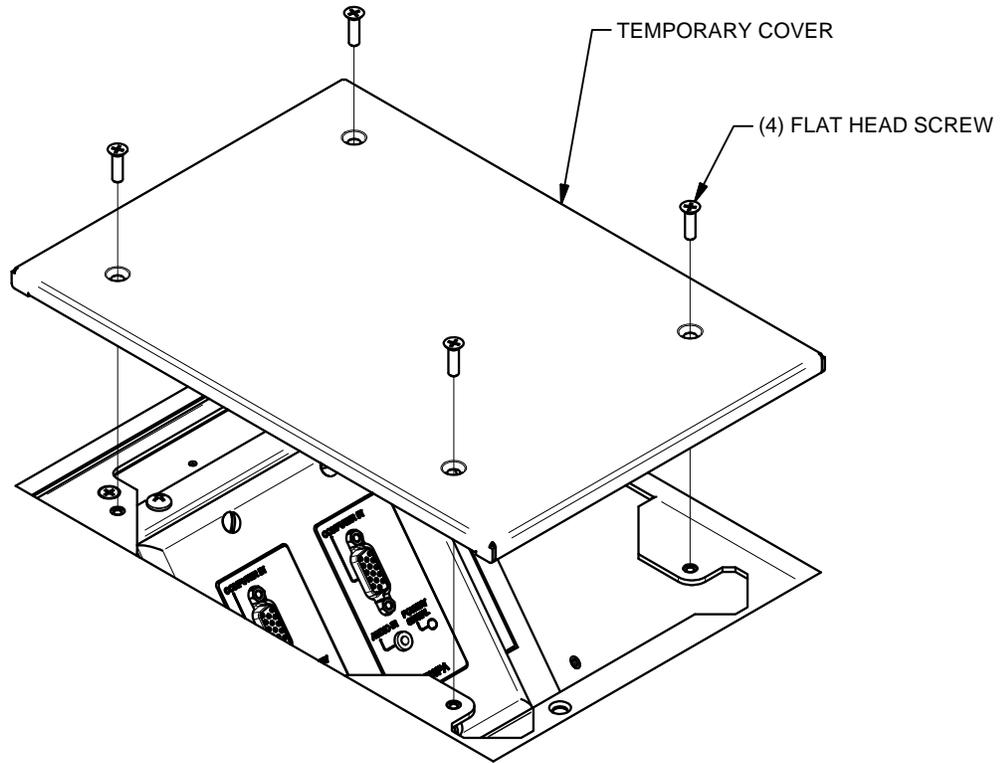
2. INSTALL CABLE INTERFACES AND CONNECTOR PLATES IF PREVIOUSLY NOT INSTALLED. CLEAN AREA IN AND AROUND ENTIRE TOP EDGE OF BOX AND APPLY 1/4" CONTINUOUS BEAD OF RTV SILICONE SEALANT.
