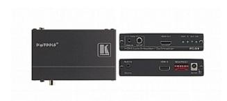
The FC-69 is a high-performance Ultra-HD (4K) HDMI audio embedder and de-embedder. The unit can embed analog audio to the HDMI output or de-embed audio from the HDMI input or from the HDMI output Audio Return Channel to S/PDIF and unbalanced stereo audio outputs simultaneously.
