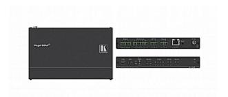
The FC-28 is a bidirectional RS-232, IR control, GPI/O and relay control signal converter to Ethernet. Two RS-232, four IR, two GPI/O and two relay controllable devices can be controlled via an Ethernet or LAN connection.
