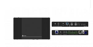
EXT3-21-XR-TR is a high-performance, extended-reach HDBaseT 3.0 extender for 4K60Hz (4:4:4) HDMI, USB, Ethernet, RS-232, and IR signals over twisted pair, flexibly set as transmitter-side or receiver-side device.
