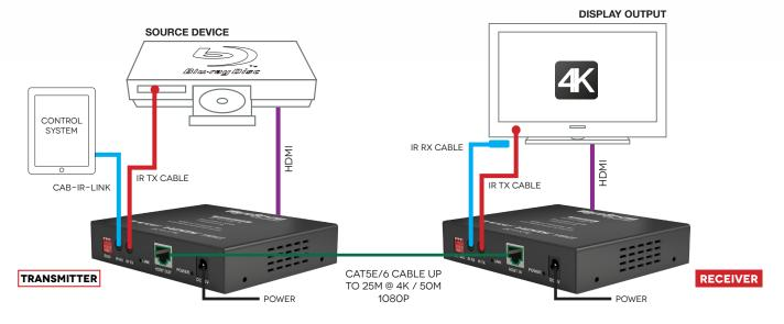
NOTE: HDMI cable length should not exceed 10m/33ft. HD LED/plasma displays can also be substituted for any other HDMI display device, such as a digital projector or further extended using another WyreStorm extender set featuring alternative transmission such as fiber or UTP/HDBaseT. EXP-EX-HDBT-50 may also be integrated into a larger HDBaseT matrix distribution using HDMI input connectivity.
