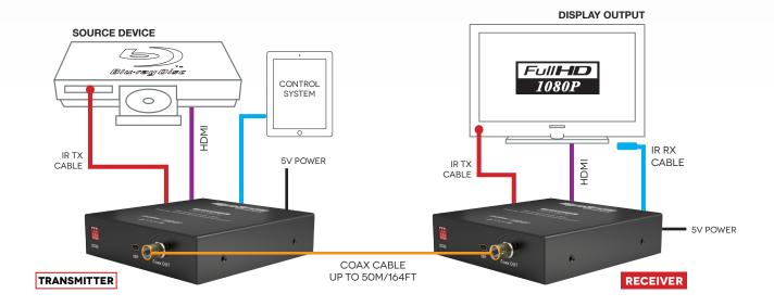
NOTE: HDMI cable length should not exceed 10m/33ft. HD LED/plasma displays can also be substituted for any other HDMI display device, such as a digital projector or further extended using another WyreStorm extender set featuring alternative transmission such as fiber or UTP/HDBaseT. EXP-EX-COAX-50 may also be integrated into a larger HDBaseT matrix distribution using HDMI input connectivity.
