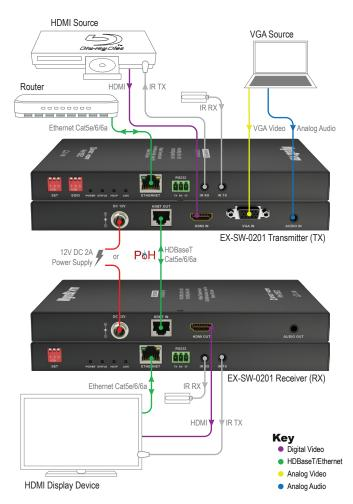
IMPORTANT! Do not connect or disconnect (hot plug) the HDMI, or HDBaseT connections while the transmitter or receiver is powered on. Doing so may cause damage to the units or connected devices.
