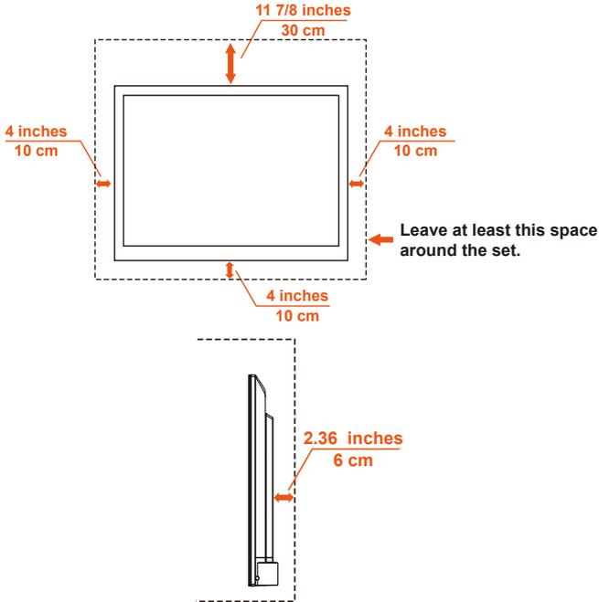
For use only with UL Listed Wall Mount Bracket with minimum weight / load:
