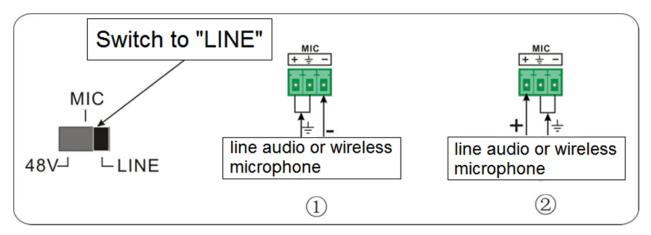
2. Balanced connection: "+" connects to positive, "-" connects to negative and "\(\ddot\)" connects to ground.
