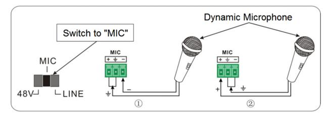
2) Balanced connection: "+" connects to positive, "-" connects to negative and "=" connects to ground.
