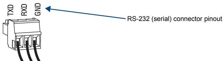
FIG. 34 Wire RS-232 ports for serial data transfer
