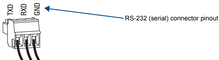
FIG. 34 Wire RS-232 ports for serial data transfer
