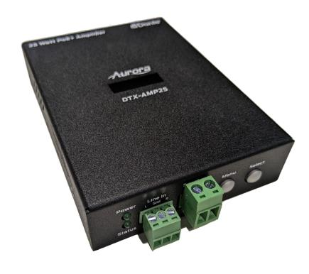
The DTX-AMP25-M is a 25-Watt PoE+ Dante amplifier allowing audio distribution of small to very large scale. The small form factor and light weight allows it to be mounted just about anywhere. The 4/8 Ohm out can drive 2 speakers in parallel saving cost. It also features an OLED for IP Address and other status information for better setup and serviceability.
