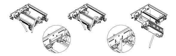
To remove and reassemble power units from grommet assembly. Note: For corded version only.
