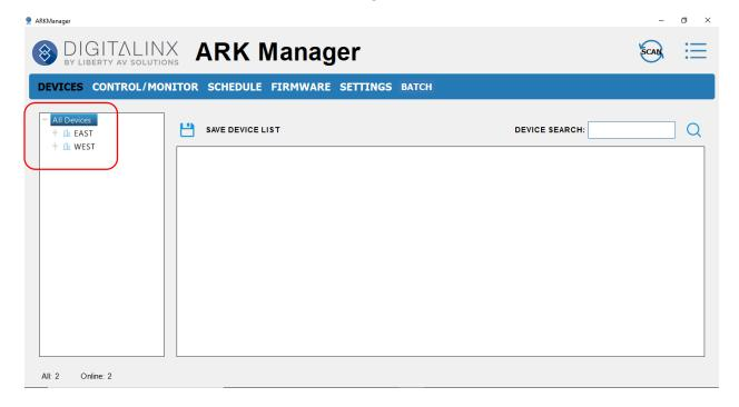
Click on the building, floor to view the room number assigned to the DL-ARK device. In our example system we have configured two systems, one resides in room 101 on Floor 1 in the EAST building and one resides in room 102 on Floor 1 of the WEST building.
