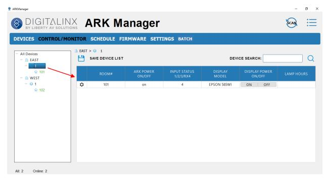
**NOTE:** In order to see current display status, turn display on/off and see current lamp hours in this quick view list, the DL-ARK must be configured first with the preferred control protocol and proper commands. For detailed control configuration set up, reference the DL-ARK Deployment Guide on page 31 and 32.
