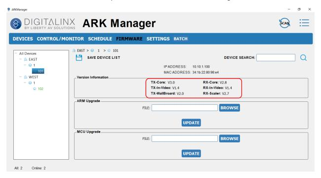
NOTE: Firmware can also be uploaded en masse using the BATCH menu
