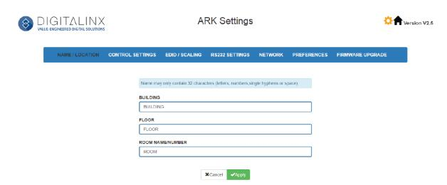
In this menu the device can organized into a building, floor and room naming convention. Enter in the desired building, floor and room identification and click *APPLY*.
