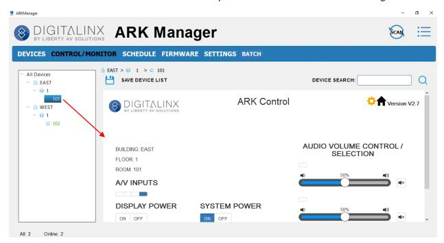
The *CONTROL/MONITOR* option uses the internal built in GUI for the selected device to control or configure said device. For detailed system configuration reference the DL-ARK Deployment Guide on page 27.
