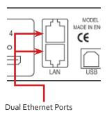
Connect the Fx4 to a network using the top LAN connector then open Wall Designer and create your display layout. At the point where you associate the virtual device with a physical device the list will display all Fx4's currently connected to the network either directly or daisy chained.
