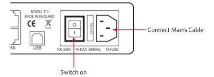
When the power is switched on the Fx4 will boot and the LEDs on the front panel will flash for up to 15 seconds. Should the LED's continue to flash see the troubleshooting section.
