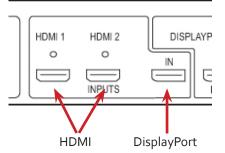
Connect your input source to one of the 3 input connectors on the rear of the Fx4. You can connect up to 3 input sources, 2 x HDMI and 1 x DisplayPort.
