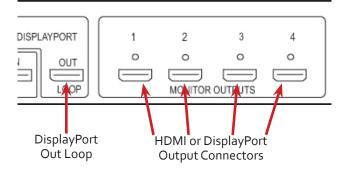
Connect the monitor cables to the monitor output connectors on the rear of the Fx4, you can connect up to 4 monitors to a single Fx4 unit. Ensure the cables are inserted correctly, it is recommended that locking connectors are used.
