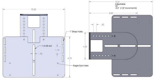
AVF's **CS** wall mounted camera or codec shelf is designed as a two (2) piece system for either camera or video conference codec with room for adjustments. Holes for on-wall or in-wall wiring channel.
