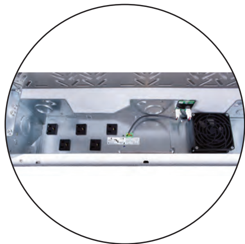
Temperature-controlled variable speed fan kit (Factory Installed in CB-22S+ and CB-22SP+) Fan turns on at minimum speed at 29° C Fan reaches maximum speed at 40° C Cooling capacity is approximately 150 watts/ 500 BTU/hr with a 10° temperature rise above ambient.
