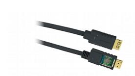
CA-HM active HDMI copper cable provides a perfect cable solution for delivering HDMI signals over long distances: 18Gbps up to 20m (66ft), 10.2 Gbps up to 25m (82ft) and 6.75Gbps up to 30m (98ft). The innovative technology utilized in the cable's connector features superior equalizing and signal compensation to meet the most demanding challenges in Pro AV installations.
