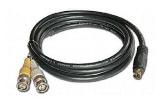
Kramer's s-Video (Y/C) breakout cable is constructed of dual mini coax cables with a male s-Video (4-pin) connector on one end and 2 BNCs on the other. They are used for converting an s-Video signal from the typical 4-pin format to higher quality dual BNC format preferred for long cable runs.
