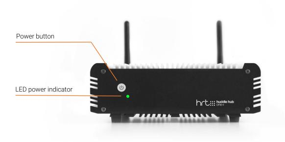
HHO powers on automatically when connected to the wall socket. The LED power indicator on the front panels turns from red to green.
