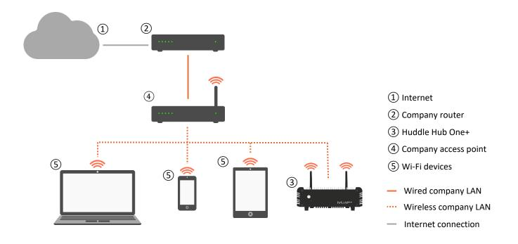
Station mode is useful when you have no way to connect HHO+ to the company LAN with an Ethernet cable. In this configuration, HHO+(3) is connected to the company LAN via its Wi-Fi module, through an access point (4), as the devices (5) do.
