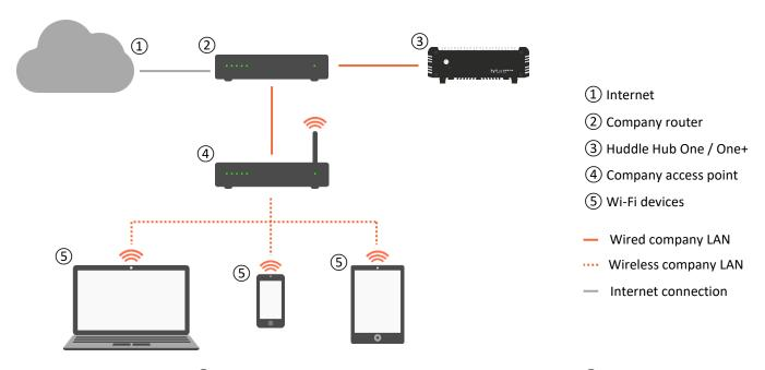
In this configuration, HHO ③ is connected to the company LAN. The Wi-Fi devices ⑤ reach HHO through a company access point ④.
