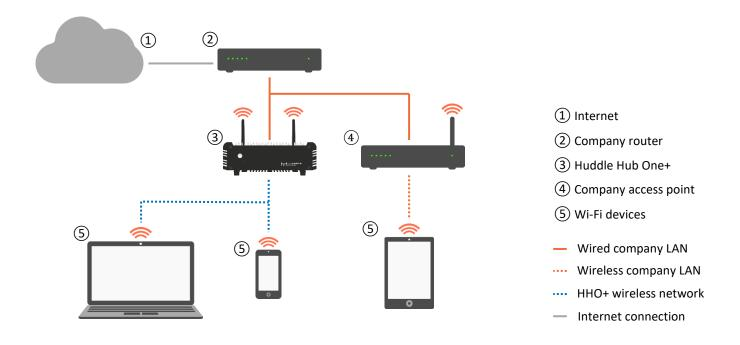
In a mixed configuration, part of the devices (5) reach HHO+(3) via a direct connection, and another part via the company LAN through an access point (4).
