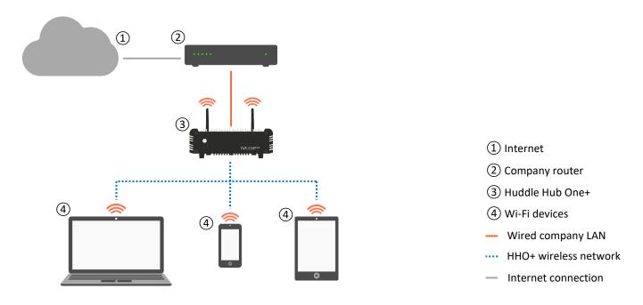
HHO+ features an on-board access point, which the Wi-Fi devices can connect to.
