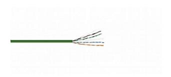
Kramer's BCLS-21 is a high-performance CAT 6 U/UTP cable designed for IT, LAN and Ethernet installations. It is constructed with four pairs of 23AWG solid bare copper conductors with a cross filler. It is enclosed in an LSZH jacket with internal rip cord and sequential markings every meter and packed in a Reelex II carton for easy to pull-out. BCLS-21 cable exceeds CAT 6 specifications to provide additional performance and bandwidth beyond the basic standard.
