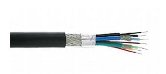
Kramer's BC-5X5S is a high-resolution, 28AWG  $75\Omega$  5 mini-coaxial cable with 5 additional 28AWG single strands and an outer shield. Its unique design is ideal for building into 5 BNC or 15-pin HD (VGA/UXGA) cables and routing computer graphic video signals in professional AV systems.
