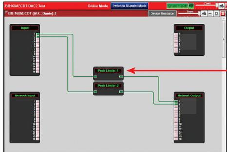
**Note:** Always add a limiter before the network output. Set the limiter threshold to 0dBu to prevent clipping the input of the HPA amplifier.
