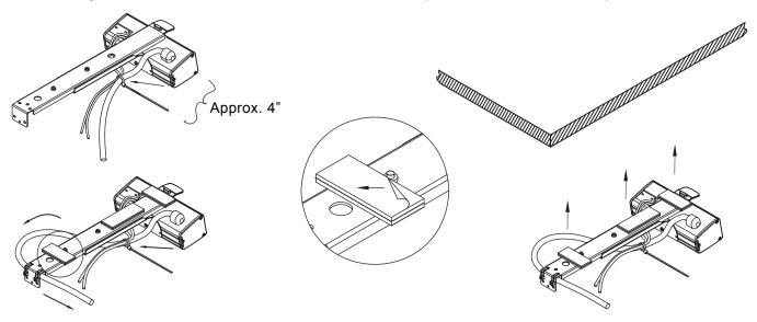
With unit fully extended, attach data cables to the power cord or top channel
