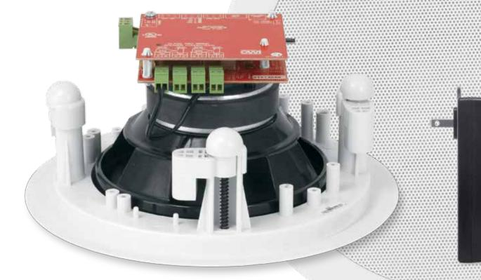
The OWI AMP-R2SIC5 / AMP-R2SIC6 is a self-powered speaker / amplifier. This amplifier can drive up to four speakers connected series parallel to have a net impedance of 8 Ohms. With an included UL Listed, Level 🕥 (Energy Star), power supply, the amplifier can output 40 watts or 10 watts per speaker in a four speaker hook-up.
