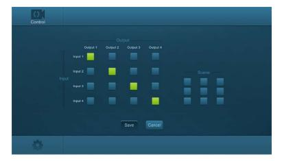
The button matrix displays every possible connection between every input and output, users can carry on the connections by clicking corresponding button.
