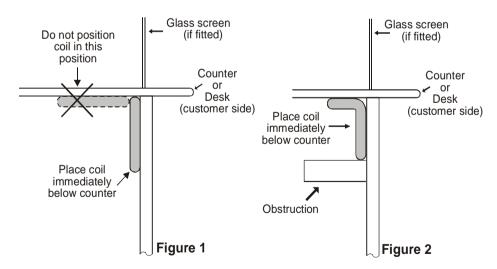
Position the loop coil as shown in **Figure 1**, with the larger dimension of the coil horizontal.
