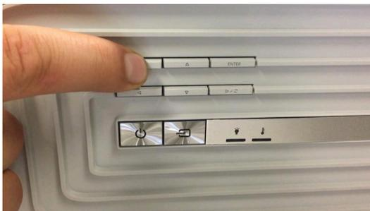
2. While continuing to hold down the menu button, reconnect the power plug to the projector.
