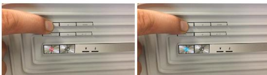
3. Once the Power LED switch to a flashing blue LED only, IMMEDIATELY let go of the menu button and wait until you see the power LED flash purple. Once it is purple, IMMEDIATELY press the menu button once.
