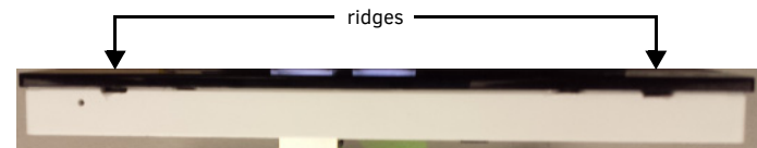
FIG. 5 LOCATION OF RIDGES ON BOTTOM OF MKP-108
