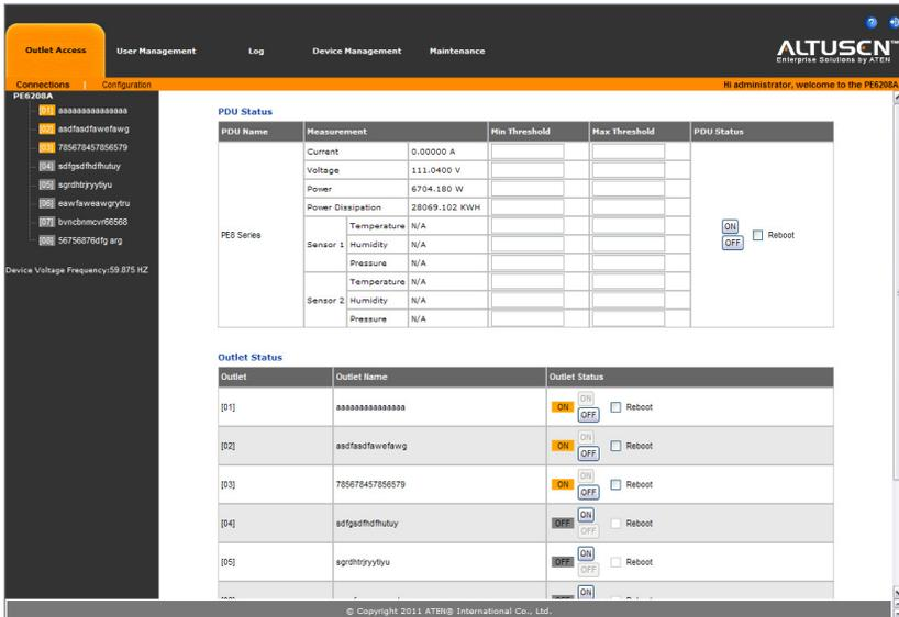
**Note:** Only enabled eco PDU models will display the Outlet Status submenu section. Other models provide only PDU Status monitoring. See *PE Series eco PDU Comparison Chart*, page 3, for which models support PDU and Outlet Status or PDU Status only monitoring.
