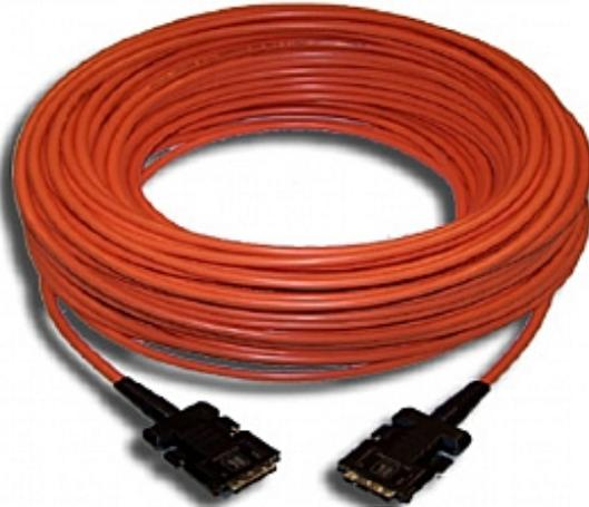
Kramer's all DVI cable system is constructed of high-performance hybrid cable containing fiber optic and copper wires terminated with DVI-D connectors on each end. They are designed to transmit DVI-D signals extremely long distances with pristine digital image quality video with the copper cable carrying additional data required for HDCP compliance.
