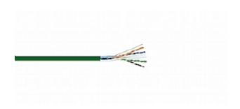
Kramer's BCLS-23 is a high-performance CAT 6 F/UTP cable designed for IT, LAN and Ethernet installations. The cable is constructed with 23AWG solid bare copper conductors with a cross filler and overall metal foil screen with a drain wire. It is enclosed in an LSZH jacket with sequential markings every meter and packed on a fumigated plywood reel. BCLS-23 cable exceeds CAT 6 specifications to provide additional performance and bandwidth beyond the basic standard.
