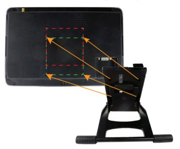
The mount has screw holes for both 75 mm x 75 mm, and 100 mm x 100 mm VESA standards, but the Touch Panel Controller only has 75 mm x 75 mm mounting holes.
