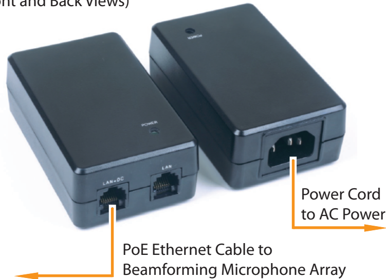
Power Over Ethernet (PoE) Power Supply (Front and Back Views)
